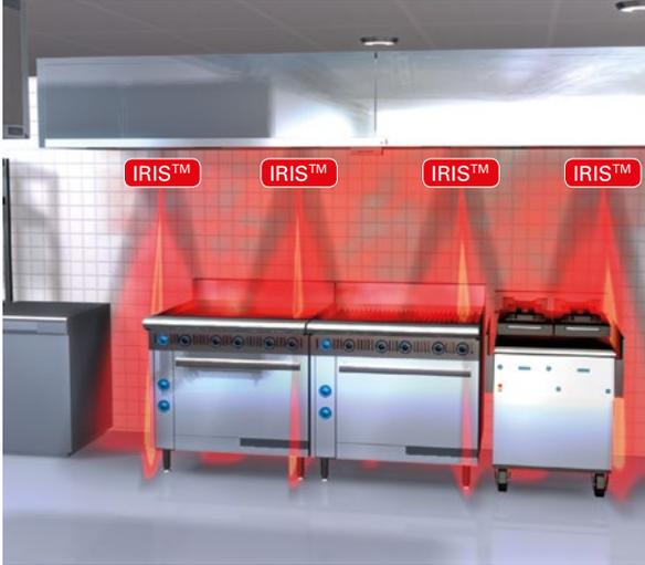
IRIS™ sensors were developed for real-time measurement and control of the thermal signature of each type of cooking appliance. They emit a beam that can instantaneously measure changes in the surface temperature of the kitchen equipment. The sensors are controlled by our special algorithm that rapidly determines when the Cold Mist has to be activated. Heat and pollutants generated by the cooking activities are then treated efficiently and appropriately with the lowest water consumption.
